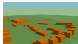
Level of Detail 1 (LoD1), Klötzchenmodell
